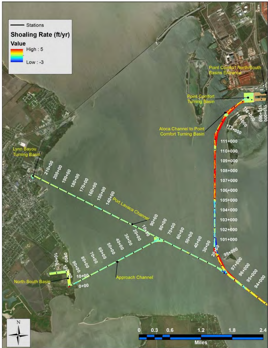
Figure 8. Map showing the shoaling rates for the part of Light 48 to Alcoa Channel reach (station 65+000 to station 110+000): Approach Channel, North-South Basin, Port Lavaca Channel, Lynn Bayou Turning Basin, Alcoa Channel to Point Comfort Turning Basin, Point Comfort Turning Basin, and Point Comfort North/South Basin Entrance. The red color signifies areas of higher shoaling, while blue color denotes erosion areas. Black lines denote station location along the reach.
