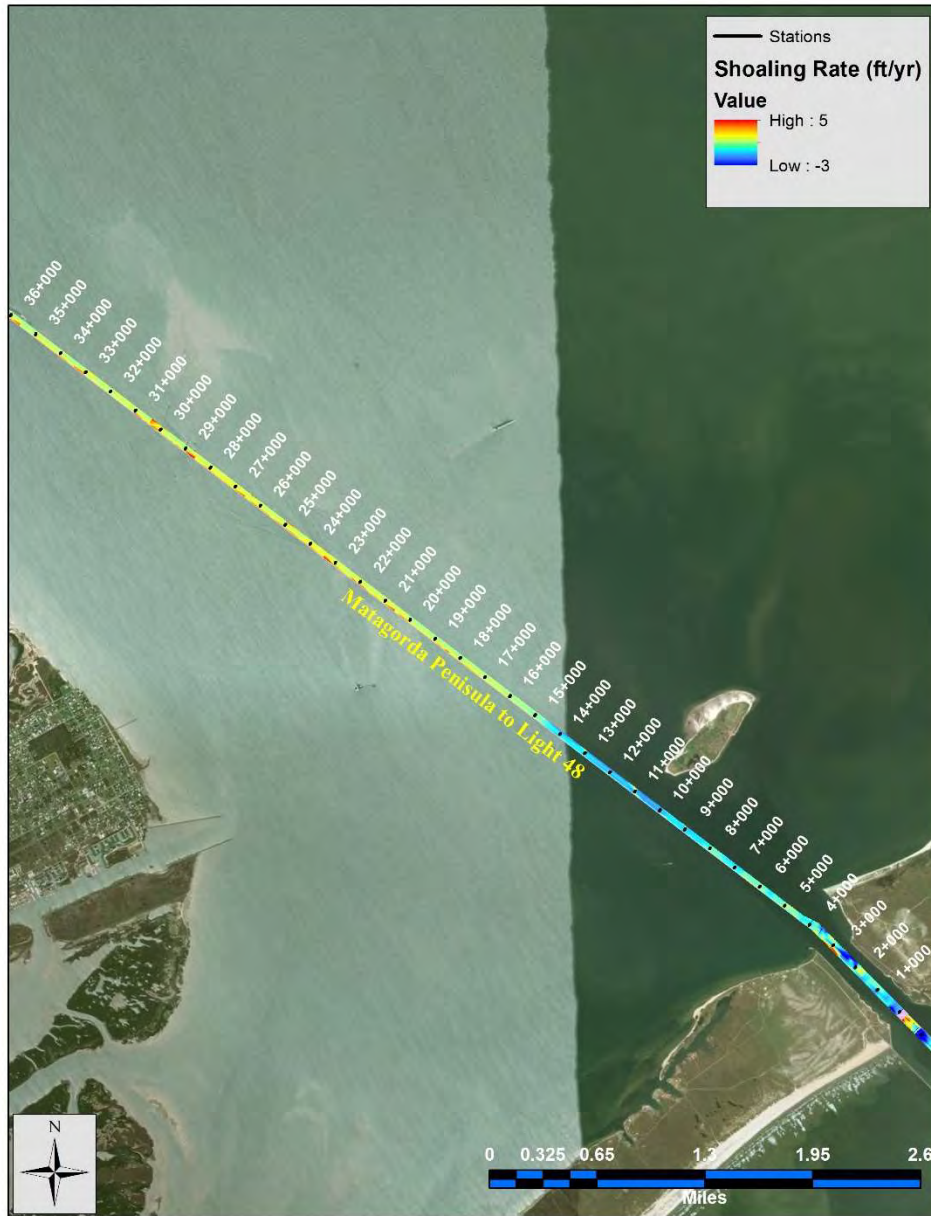
Figure 5. Map showing the shoaling rates for the part of Matagorda Peninsula to Light 48 channel reach (station 0+000 to station 36+000): The red color signifies areas of higher shoaling, while blue color denotes erosion areas. Black lines denote station locations along the reach.
