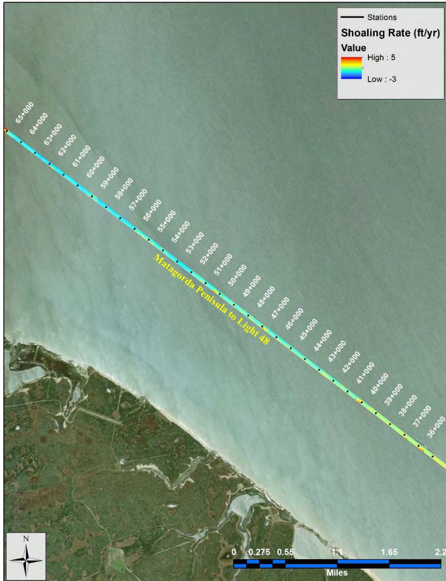
Figure 6. Map showing the shoaling rates for the part of Matagorda Peninsula to Light 48 channel reach (station 36+000 to station 65+000): The red color signifies areas of higher shoaling, while blue color denotes erosion areas. Black lines denote station location along the reach.
